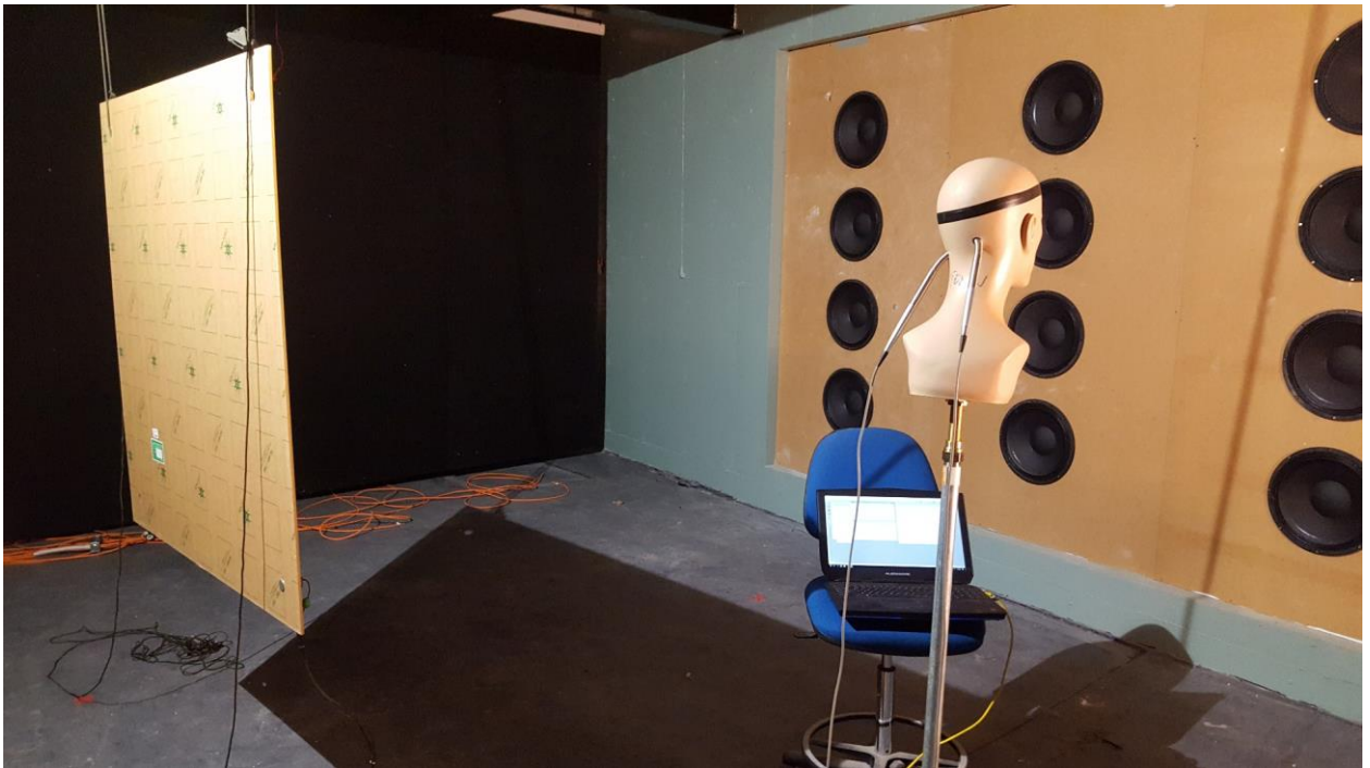
Figure 5: Manikin at RHS hotspot set at 0^\circ position (facing speaker baffle)
